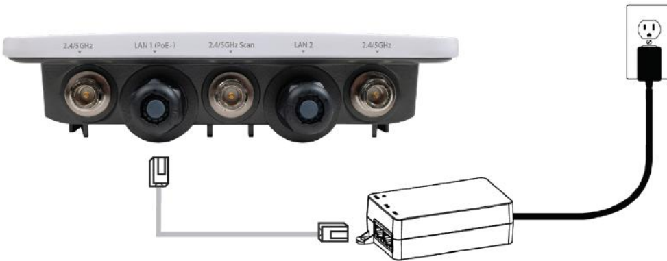
Access Point connected to PoE+ injector
